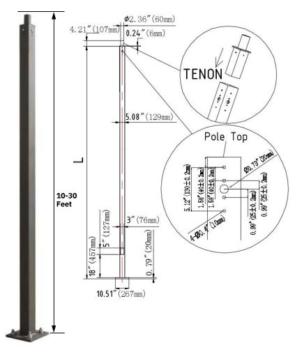
The United Pole Products Series Square aluminum poles are built from high strength aluminum Square tube and are available side drilled for arm mounted area lighting luminaires or with tenon mounts for flood and post top luminaires. Typical area lighting applications include retail centers, industrial parks, schools and universities, public transit and airports, office buildings and medical facilities. Mounting heights of 10 to 30 feet can be used based on selected luminaire application.
