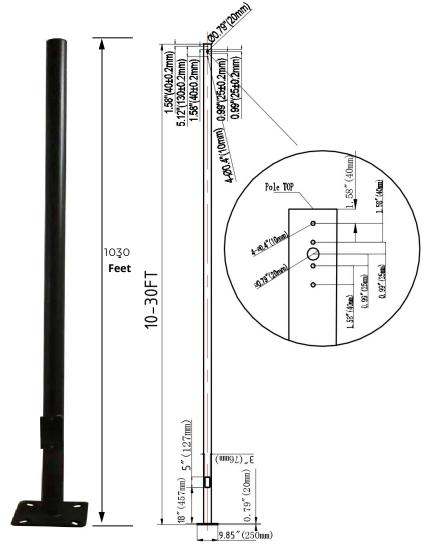
The United Pole Products Series Round aluminum poles are built from high strength aluminum Round tube and are available side drilled for arm mounted area lighting luminaires or with tenon mounts for flood and post top luminaires. Typical area lighting applications include retail centers, industrial parks, schools and universities, public transit and airports, office buildings and medical facilities. Mounting heights of 10 to 30 feet can be used based on selected luminaire application.
