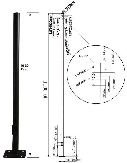
The United Pole Products Series Round Steel poles are built from high strength Steel Round tube and are available side drilled for arm mounted area lighting luminaires or with tenon mounts for flood and post top luminaires. Typical area lighting applications include retail centers, industrial parks, schools and universities, public transit and airports, office buildings and medical facilities. Mounting heights of 10 to 30 feet can be used based on selected luminaire application.
